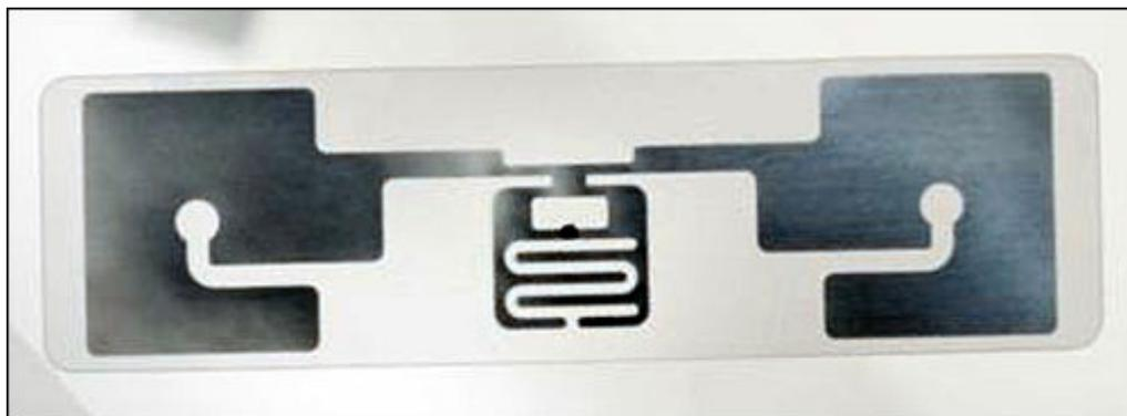
The Sensor DogBone tag is made with RFMicron's Magnus S Sensor, a moisture-sensing passive UHF RFID chip
