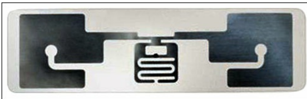
Smartrac's Sensor DogBone tag is made with RFMicron's Magnus S moisture-sensing chip.
